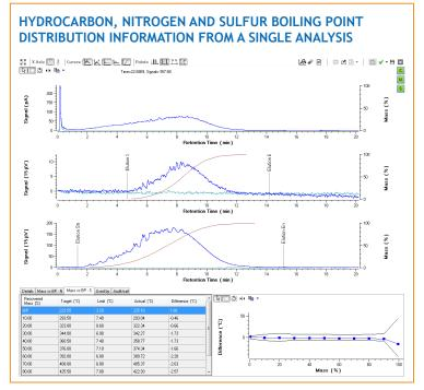
Example of a diesel sample - A single analysis run yields three chromatograms
